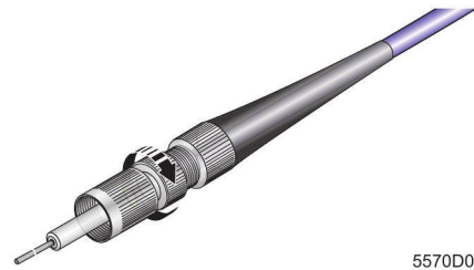
Figure 40 Screwing on the basic unit (with the example of an F-SMA connector)
